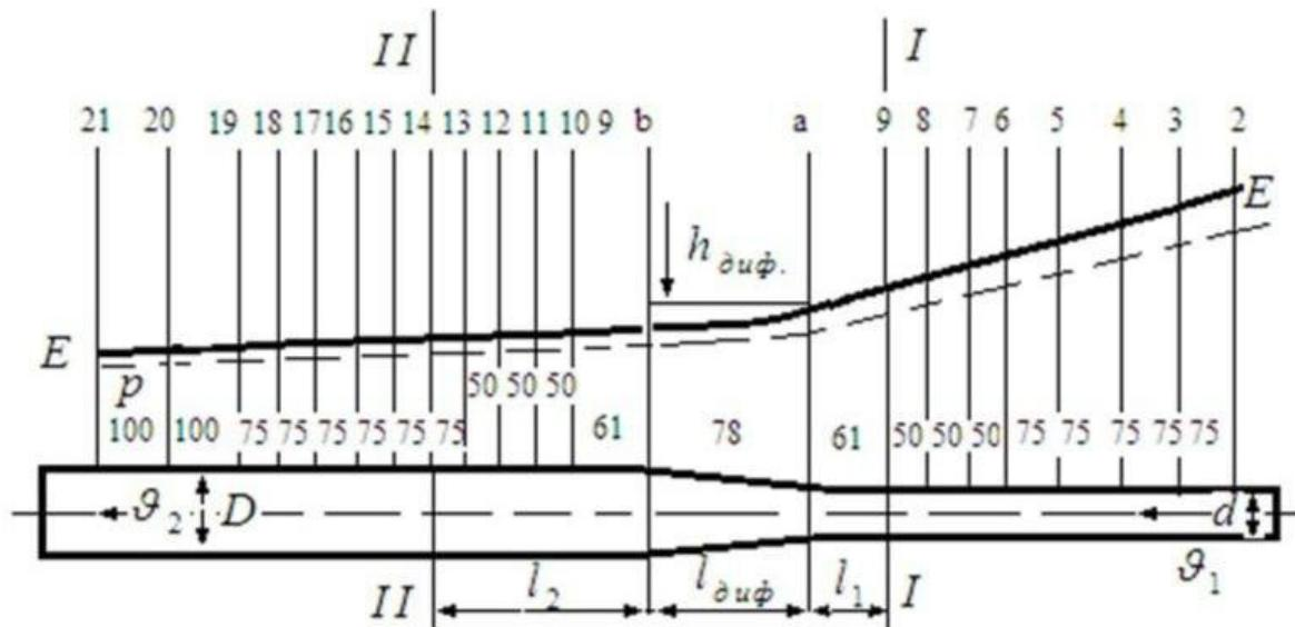
Figure 1. Diagram for determining pressure losses in a diffuser
