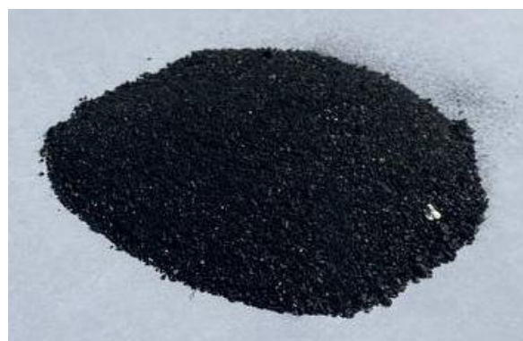
Figure 4. Type of slag produced from a reverberatory smelting furnace, before grinding (a) and after grinding (b).
