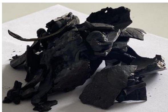
Figure 4. Type of slag produced from a reverberatory smelting furnace, before grinding (a) and after grinding (b).
