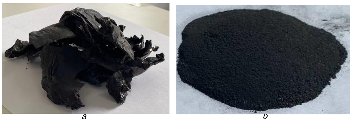
Figure 2. Type of slag formed from the Vanyukov furnace, before grinding ( a ) and after grinding ( b ).
