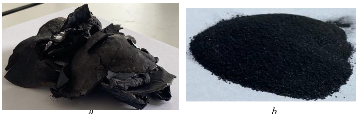
Figure 3. Type of slag formed from the OFM, before grinding ( a ) and after grinding ( b ).
