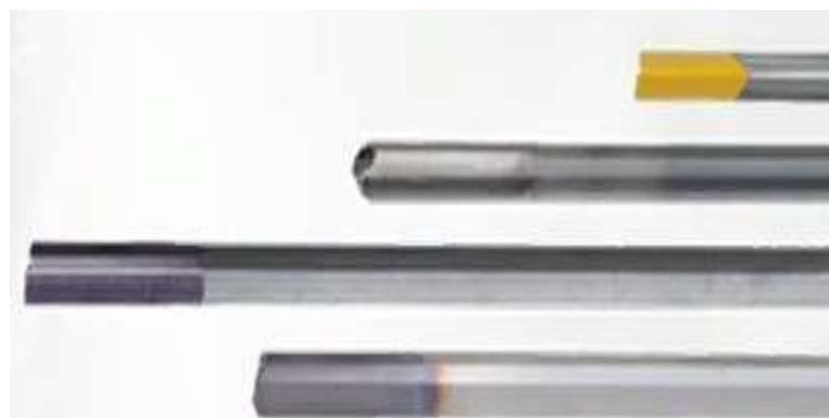
Fig. 1. Gun drills with coatings deposited
