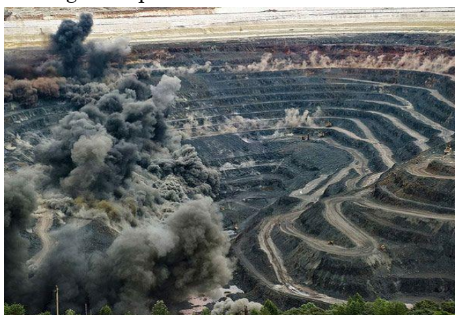
Figure 1. Explosive process in the quarry, toxic substances spreading into the air.
