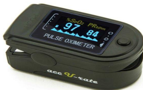
Figure No. (1) A device that measures the percentage of oxygen saturation in the blood and measures the number of heart beats per minute (Oximeter).
