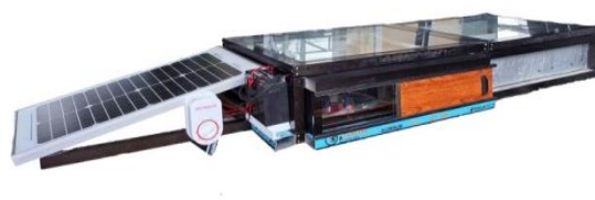
Figure 2: Multi-Functional Solar-Based Grain Storage Dryer
