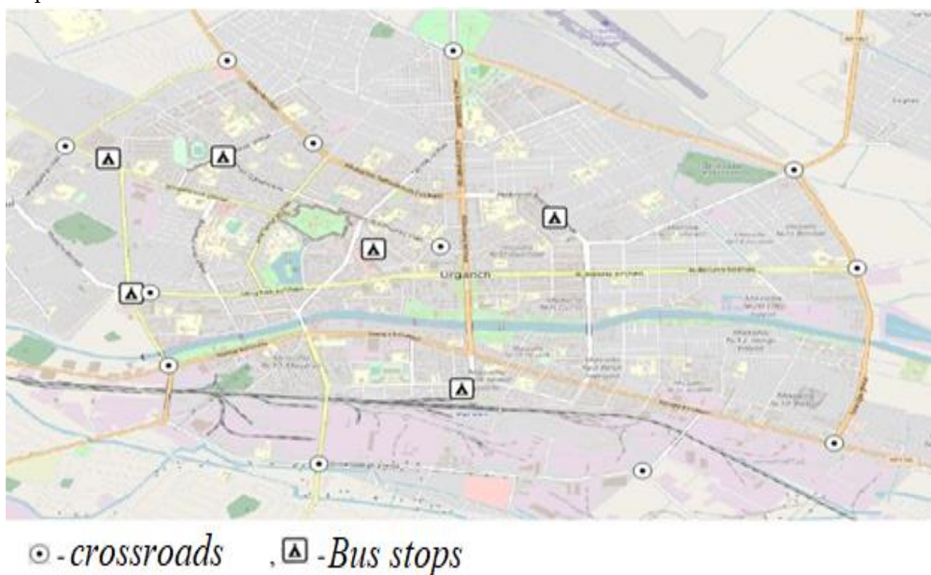
Figure-1. Address location scheme of passenger flow measurement points in public transport Enumerators standing at 12 points at road intersections visually observed public vehicles passing through the intersection, evaluated the time of passing through the intersection, the degree of occupancy of public transportation in a point system and took pictures. Enumerators at bus stops recorded the time of arrival of buses at the stop, the level of occupancy, and the number of passengers who got on and off the bus.
