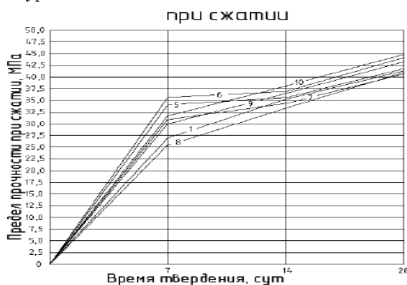
Figure 2. Influence of chemical additives on the strength of fine-grained concrete: 1 - control composition, 5 - Polyplast R 0.5% additive, 6 - Polyplast R 1% additive, 7 - Polyplast R 1.5% additive, 8 - additive Poliplast R type 2-0.5%, 9 - additive Poliplast R type 2-1%, 10 - additive Polyplast R type 2 - 1.5%.
