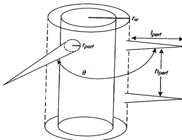
Figure-2. Well variables for perforation skin calculation (From Karakas and Tariq 1988)
