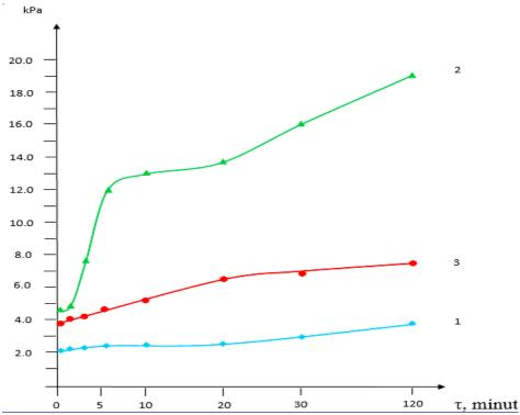
Change in plastic strength under the action of soaking 8 ml of liquid in 50 g of sand: 1) 8 ml; 2) 6ml; 3) 4 ml.
